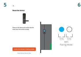
You will be prompted to reset the device (Wi-Fi Pairing Mode) press and HOLD the button for 7 Seconds to enter the WiFi Pairing Mode.
