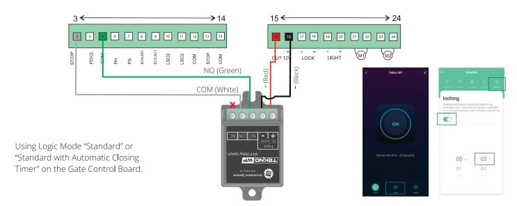
After adding the device to the APP set an "Inching" time of 02 seconds.
