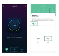
After adding the device to the APP set an "Inching" time of 02 seconds.
